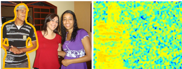
Fig. 7 An image from the CARV dataset and its output using CFA1. Darker hues correspond to lower values. The mean probability of tampering within the mask is around 0.6 while the mean outside the mask is around 0.5. However, there are many local deviations, especially with some high-value regions outside the mask
