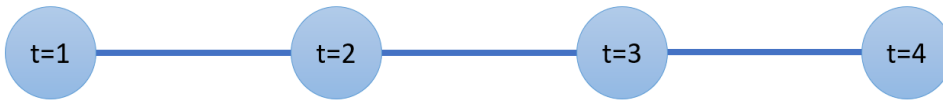
Figure 4. Viewing time as a graph. In this case, graph signal processing becomes time signal processing.
