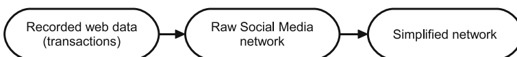
Fig. 1 Typical lifecycle of a Social Media network: A set of transactions involving users, content and meta-data lead to the formation of a “raw” Social Media network. Typically, this network is simplified before any sophisticated analysis (e.g. community detection) takes place
